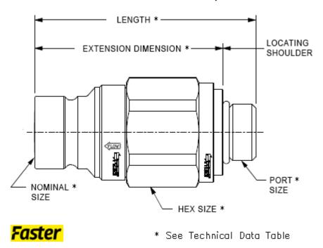
Faster FFH style, flat face couplings provide quick release connections to Sun's integrated packages, helping to prevent contamination and spillage.
