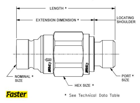
Faster FFH style, flat face couplings provide quick release connections to Sun's integrated packages, helping to prevent contamination and spillage.
