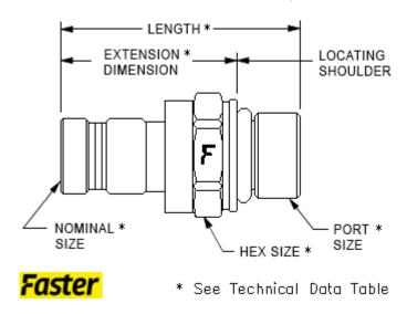
Faster flat face diagnostic couplings provide quick release access points to measure pressure within Sun's integrated packages.
