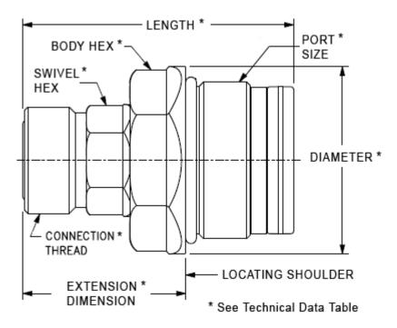
Taimi cartridge swivel fittings are designed to be integrated directly into the hydraulic manifold. When installed, the fitting provides a superior, rugged and low-profile swivel port that can withstand high pressures and side loads.
