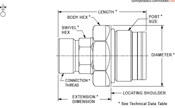
Taimi cartridge swivel fittings are designed to be integrated directly into the hydraulic manifold. When installed, the fitting provides a superior, rugged and low-profile swivel port that can withstand high pressures and side loads.
