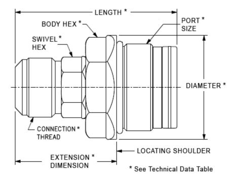
Taimi cartridge swivel fittings are designed to be integrated directly into the hydraulic manifold. When installed, the fitting provides a superior, rugged and low-profile swivel port that can withstand high pressures and side loads.
