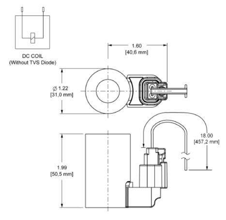
This 740 Series Coil configuration uses a connector adapter kit to provide the required termination.
