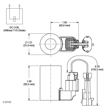
This 740 Series Coil configuration uses a connector adapter kit to provide the required termination.
