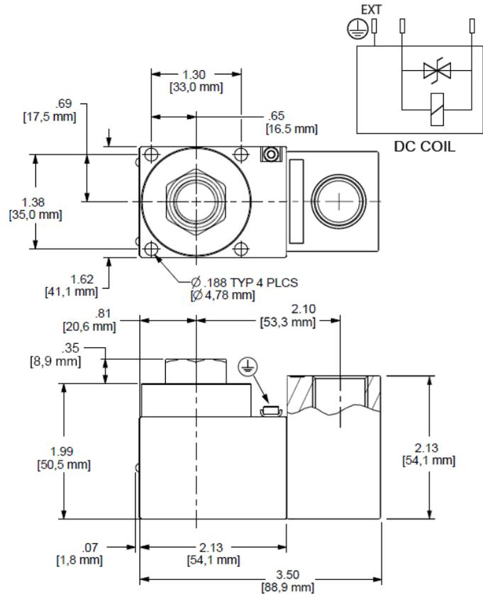
Model 747 Series hazardous location coils are designed for Sun's FLeX Series switching and proportional solenoid valves and for newer Sun valves that use the 16-mm actuator tubes. All models include ATEX, IECEX, and NEC, CEC/CSA certifications.
