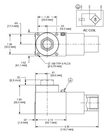
Model 747 Series hazardous location coils are designed for Sun's FLeX Series switching and proportional solenoid valves and for newer Sun valves that use the 16-mm actuator tubes. All models include ATEX, IECEx, and NEC, CEC/CSA certifications.
