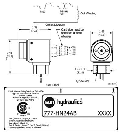
Sun offers explosion proof coils for use in hazardous environments. Certification requires the explosion proof coil to be sold as a complete cartridge/coil assembly. Coil cannot be purchased separately. For ordering information, please see the coil option section on the applicable cartridge product page.
