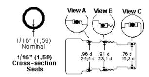
Sun offers replacement seal kits for all cartridge models. These kits include all of the external seals on the cartridge along with installation instructions. Seal kits are available in Buna-N and Viton for all models, along with EPDM and polyurethane for many models. Please note: Converting the external seals from one material to another does not ensure fluid compatibility with that material due to the existence of internal seals within the cartridge.
