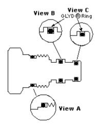
Sun offers replacement seal kits for all cartridge models. These kits include all of the external seals on the cartridge along with installation instructions. Seal kits are available in Buna-N and Viton for all models, along with EPDM and polyurethane for many models. Please note: Converting the external seals from one material to another does not ensure fluid compatibility with that material due to the existence of internal seals within the cartridge.
