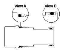
Sun offers replacement seal kits for all cartridge models. These kits include all of the external seals on the cartridge along with installation instructions. Seal kits are available in Buna-N and Viton for all models, along with EPDM and polyurethane for many models. Please note: Converting the external seals from one material to another does not ensure fluid compatibility with that material due to the existence of internal seals within the cartridge.
