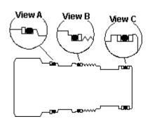
Sun offers replacement seal kits for all cartridge models. These kits include all of the external seals on the cartridge along with installation instructions. Seal kits are available in Buna-N and Viton for all models, along with EPDM and polyurethane for many models. Please note: Converting the external seals from one material to another does not ensure fluid compatibility with that material due to the existence of internal seals within the cartridge.
