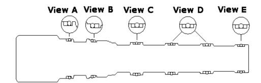
Sun offers replacement seal kits for all cartridge models. These kits include all of the external seals on the cartridge along with installation instructions. Seal kits are available in Buna-N and Viton for all models, along with EPDM and polyurethane for many models. Please note: Converting the external seals from one material to another does not ensure fluid compatibility with that material due to the existence of internal seals within the cartridge.
