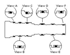
$\textbf{NOTES:} \quad \bullet \quad \text{Install back-up rings and O-rings as shown in views.}$
