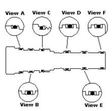
Sun offers replacement seal kits for all cartridge models. These kits include all of the external seals on the cartridge along with installation instructions. Seal kits are available in Buna-N and Viton for all models, along with EPDM and polyurethane for many models. Please note: Converting the external seals from one material to another does not ensure fluid compatibility with that material due to the existence of internal seals within the cartridge.
