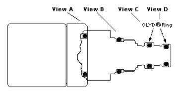
Sun offers replacement seal kits for all cartridge models. These kits include all of the external seals on the cartridge along with installation instructions. Seal kits are available in Buna-N and Viton for all models, along with EPDM and polyurethane for many models. Please note: Converting the external seals from one material to another does not ensure fluid compatibility with that material due to the existence of internal seals within the cartridge.
