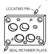
Sun ISO 07 sandwich bodies are available for many control functions and are offered in two styles. The style is determined by the method used to seal the fluid interfaces. Most of the ISO 07 sandwich bodies make use of a seal retainer plate for sealing purposes. The remaining ISO 07 bodies include counterbores in the sealing faces for O-ring installation. Seal retainer plate only, seals only, and combination kits are available.
