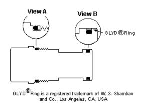
Sun offers replacement seal kits for all cartridge models. These kits include all of the external seals on the cartridge along with installation instructions. Seal kits are available in Buna-N and Viton for all models, along with EPDM and polyurethane for many models. Please note: Converting the external seals from one material to another does not ensure fluid compatibility with that material due to the existence of internal seals within the cartridge.
