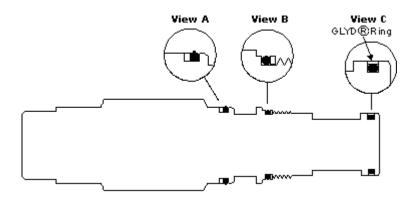
Sun offers replacement seal kits for all cartridge models. These kits include all of the external seals on the cartridge along with installation instructions. Seal kits are available in Buna-N and Viton for all models, along with EPDM and polyurethane for many models. Please note: Converting the external seals from one material to another does not ensure fluid compatibility with that material due to the existence of internal seals within the cartridge.
