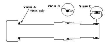
Sun offers replacement seal kits for all cartridge models. These kits include all of the external seals on the cartridge along with installation instructions. Seal kits are available in Buna-N and Viton for all models, along with EPDM and polyurethane for many models. Please note: Converting the external seals from one material to another does not ensure fluid compatibility with that material due to the existence of internal seals within the cartridge.
