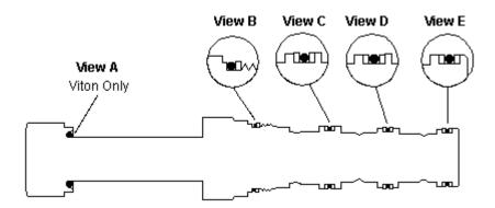
Sun offers replacement seal kits for all cartridge models. These kits include all of the external seals on the cartridge along with installation instructions. Seal kits are available in Buna-N and Viton for all models, along with EPDM and polyurethane for many models. Please note: Converting the external seals from one material to another does not ensure fluid compatibility with that material due to the existence of internal seals within the cartridge.
