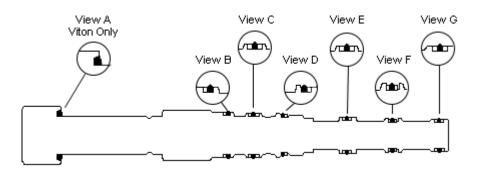
Sun offers replacement seal kits for all cartridge models. These kits include all of the external seals on the cartridge along with installation instructions. Seal kits are available in Buna-N and Viton for all models, along with EPDM and polyurethane for many models. Please note: Converting the external seals from one material to another does not ensure fluid compatibility with that material due to the existence of internal seals within the cartridge.
