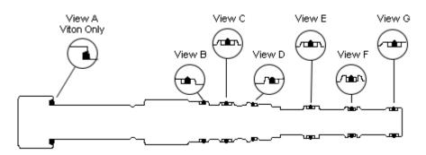
Sun offers replacement seal kits for all cartridge models. These kits include all of the external seals on the cartridge along with installation instructions. Seal kits are available in Buna-N and Viton for all models, along with EPDM and polyurethane for many models. Please note: Converting the external seals from one material to another does not ensure fluid compatibility with that material due to the existence of internal seals within the cartridge.
