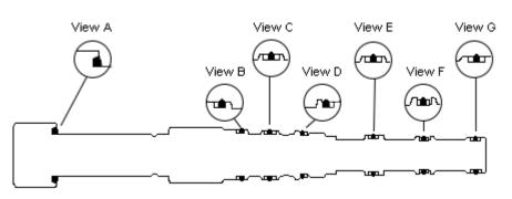
Sun offers replacement seal kits for all cartridge models. These kits include all of the external seals on the cartridge along with installation instructions. Seal kits are available in Buna-N and Viton for all models, along with EPDM and polyurethane for many models. Please note: Converting the external seals from one material to another does not ensure fluid compatibility with that material due to the existence of internal seals within the cartridge.
