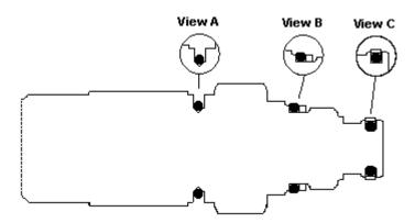
Sun offers replacement seal kits for all cartridge models. These kits include all of the external seals on the cartridge along with installation instructions. Seal kits are available in Buna-N and Viton for all models, along with EPDM and polyurethane for many models. Please note: Converting the external seals from one material to another does not ensure fluid compatibility with that material due to the existence of internal seals within the cartridge.
