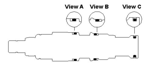
Sun offers replacement seal kits for all cartridge models. These kits include all of the external seals on the cartridge along with installation instructions. Seal kits are available in Buna-N and Viton for all models, along with EPDM and polyurethane for many models. Please note: Converting the external seals from one material to another does not ensure fluid compatibility with that material due to the existence of internal seals within the cartridge.
