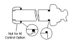
Sun coil seal kits for pilot cartridges that fit into T-8A and T-9A cavities contain all replacement seals, a replacement nut and installation instructions. Please note: all seals contained in a coil seal kit are constructed of Viton.
