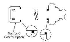
Sun coil seal kits for pilot cartridges that fit into T-8A and T-9A cavities contain all replacement seals, a replacement nut and installation instructions. Please note: all seals contained in a coil seal kit are constructed of Viton.
