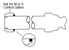
Sun coil seal kits for full flow and proportional solenoid operated cartridges contain all replacement seals, a replacement coil nut and installation instructions. Please note: All seals contained in a coil seal kit are constructed of Viton.
