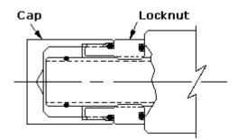
This control kit includes a removable sealed cap for protecting the adjustment screw. It is like the R Control but without the lockwire.
