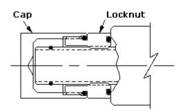
This control kit includes a removable sealed cap for protecting the adjustment screw. It is like the R Control but without the lockwire.
