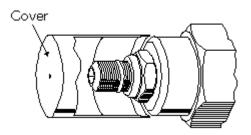
Sun's tamper resistant cover is a zinc plated steel cover which press-fits onto the L Control cartridge shoulder. Valves may be ordered in this configuration from Sun by specifying a C control in the model number. The pressure setting must be specified at the time of the order and the setting will be stamped on the cartridge hex. Sun kits for replacement parts or field conversion are available.
