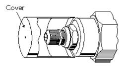
Sun's tamper resistant cover is a stainless steel cover which press-fits onto the L Control cartridge shoulder. Stainless steel cartridges only may be ordered in this configuration from Sun by specifying a C control in the model number. The pressure setting must be specified at the time of the order and the setting will be stamped on the cartridge hex. Sun kits for replacement parts or field conversion are available.
