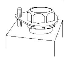
NOTES: • Tighten set screw until knurled point is firmly embedded in valve manifold/body (12-15 lb-in).
