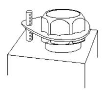
**NOTES:** • Tighten set screw until knurled point is firmly embedded in valve manifold/body (12-15 lb-in).
