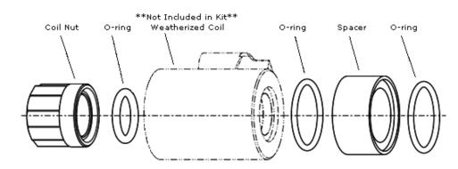
This weatherization kit is used in conjunction with a weatherized coil and a modified cavity (see below). The coil is not included in the kit and must be purchased separately. Weatherization kits are cartridge model code dependent. This kit is intended for new installations only and is not suitable for retrofitting existing equipment, or for standard Sun bodies. A selection of special line mount bodies for use in weatherized assemblies are available.
