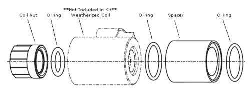
This weatherization kit is used in conjunction with a weatherized coil and a modified cavity (see below). The coil is not included in the kit and must be purchased separately. Weatherization kits are cartridge model code dependent. This kit is intended for new installations only and is not suitable for retrofitting existing equipment, or for standard Sun bodies. A selection of special line mount bodies for use in weatherized assemblies are available.
