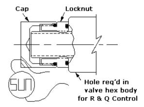
Sun offers an R control replacement kit with the added benefit of maintaining min/max setting. This kit includes a sealed cap with lockwire and a stop ring where applicable. This kit can also be used to replace a J, M, and Q control.
