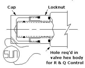
Sun offers an R control replacement kit with the added benefit of maintaining min/max setting. This kit includes a sealed cap with lockwire and a stop ring where applicable. This kit can also be used to replace a J, M, and Q control.
