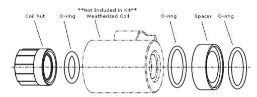
This weatherization kit is used in conjunction with a weatherized coil and a modified cavity (see below). The coil is not included in the kit and must be purchased separately. Weatherization kits are cartridge model code dependent. This kit is intended for new installations only and is not suitable for retrofitting existing equipment, or for standard Sun bodies. A selection of special line mount bodies for use in weatherized assemblies are available.
