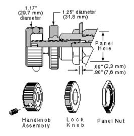
Sun offers a general purpose handknob control with panel mount nut for use in systems where the cartridge needs to be panel-mounted and frequent adjustments are necessary. The handknob components are added to the basic L control and an external thread is added to the cartridge body. Cartridges may be ordered in this configuration from Sun by specifying an O control in the model number. Sun repair kits are also available.
