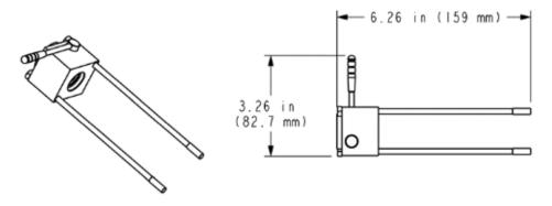
This is a momentary bi-directional, hand-actuated device for use on Sun's common cavity 3-position/4-way directional valves.
