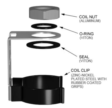
This coil clip kit is designed to attach Sun's XMD Series Driver to the FLeX low-power coil.
