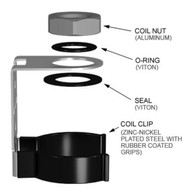
This coil clip kit is designed to attach Sun's XMD Series Driver to the FLeX low-power coil.
