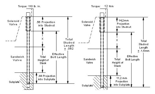
To simplify the installation of ISO 03 and ISO 05 sandwiches, Sun offers uncut (can be cut to length in the field) or precut studkits in both inch and metric standard threaded rod. Once the rods are installed in a subplate or manifold, they act as a guide in assembling the sandwich body stack. After the directional control valve is assembled on top of the stack, Sun studnuts are used to retain the assembled stack.
