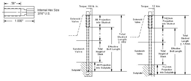
To simplify the installation of ISO 03 and ISO 05 sandwiches, Sun offers uncut (can be cut to length in the field) or precut studkits in both inch and metric standard threaded rod. Once the rods are installed in a subplate or manifold, they act as a guide in assembling the sandwich body stack. After the directional control valve is assembled on top of the stack, Sun studnuts are used to retain the assembled stack.
