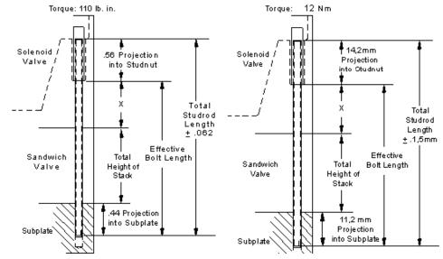
To simplify the installation of ISO 03 and ISO 05 sandwiches, Sun offers uncut (can be cut to length in the field) or precut studkits in both inch and metric standard threaded rod. Once the rods are installed in a subplate or manifold, they act as a guide in assembling the sandwich body stack. After the directional control valve is assembled on top of the stack, Sun studnuts are used to retain the assembled stack.
